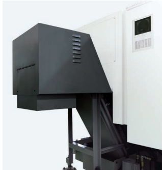
Rear discharge chip conveyor
