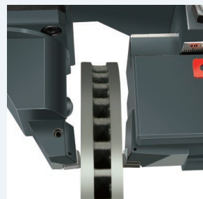
Simultaneous dual-face turning of disk brake
